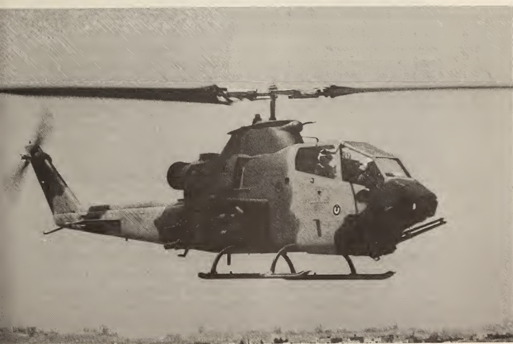
Soldier firing a mortar Cobra attack helicopter armed with TOW antitank missiles of the Royal Jordanian Air Force
